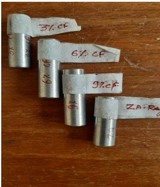
Figure 4: Produced pallets for Pin-on-Disc Testing
