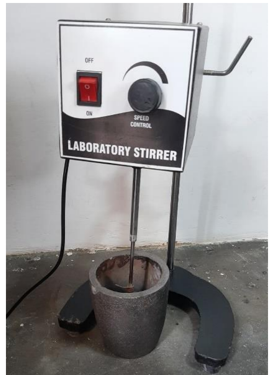
Figure 1: Laboratory Stirrer for homogeneous mixing of ZA27 with Carbon Fibre
