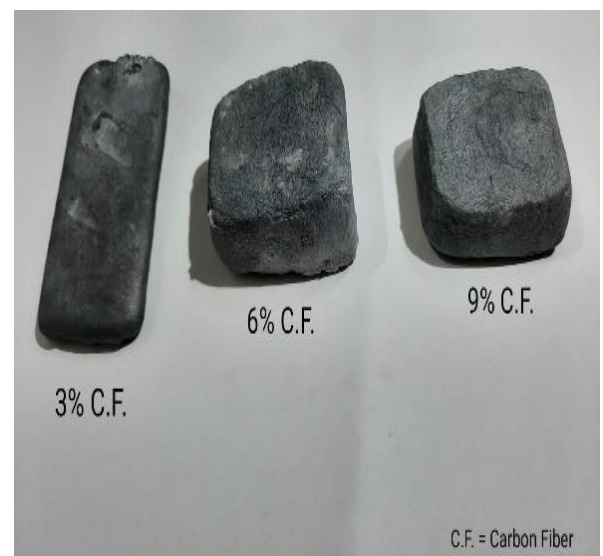
Figure 2: ZA27 reinforced with Carbon Fibre
