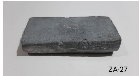
Figure 2 ZA-27 Sample prepared after Stir Casting.
