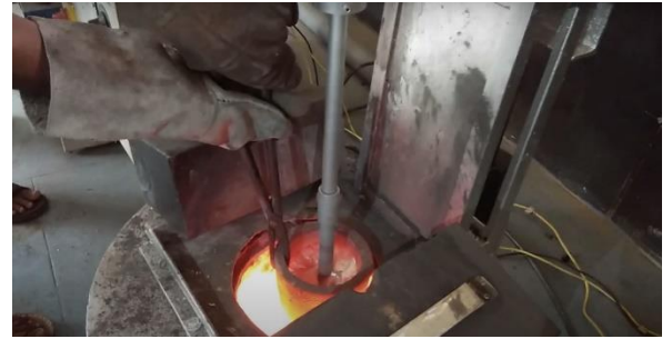
Figure 1 Stir Casting with Laboratory Stirrer
