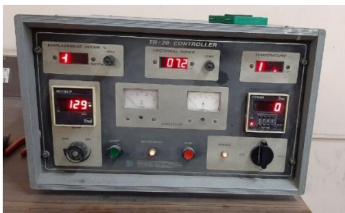
Figure 10 Digital Control Panel (Wear Test Apparatus)
