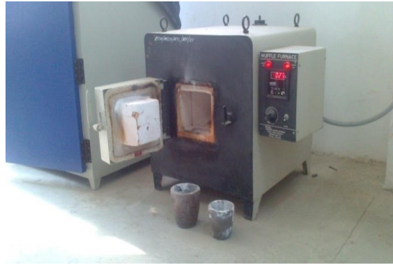
Fig-1 Muffle furnace.
